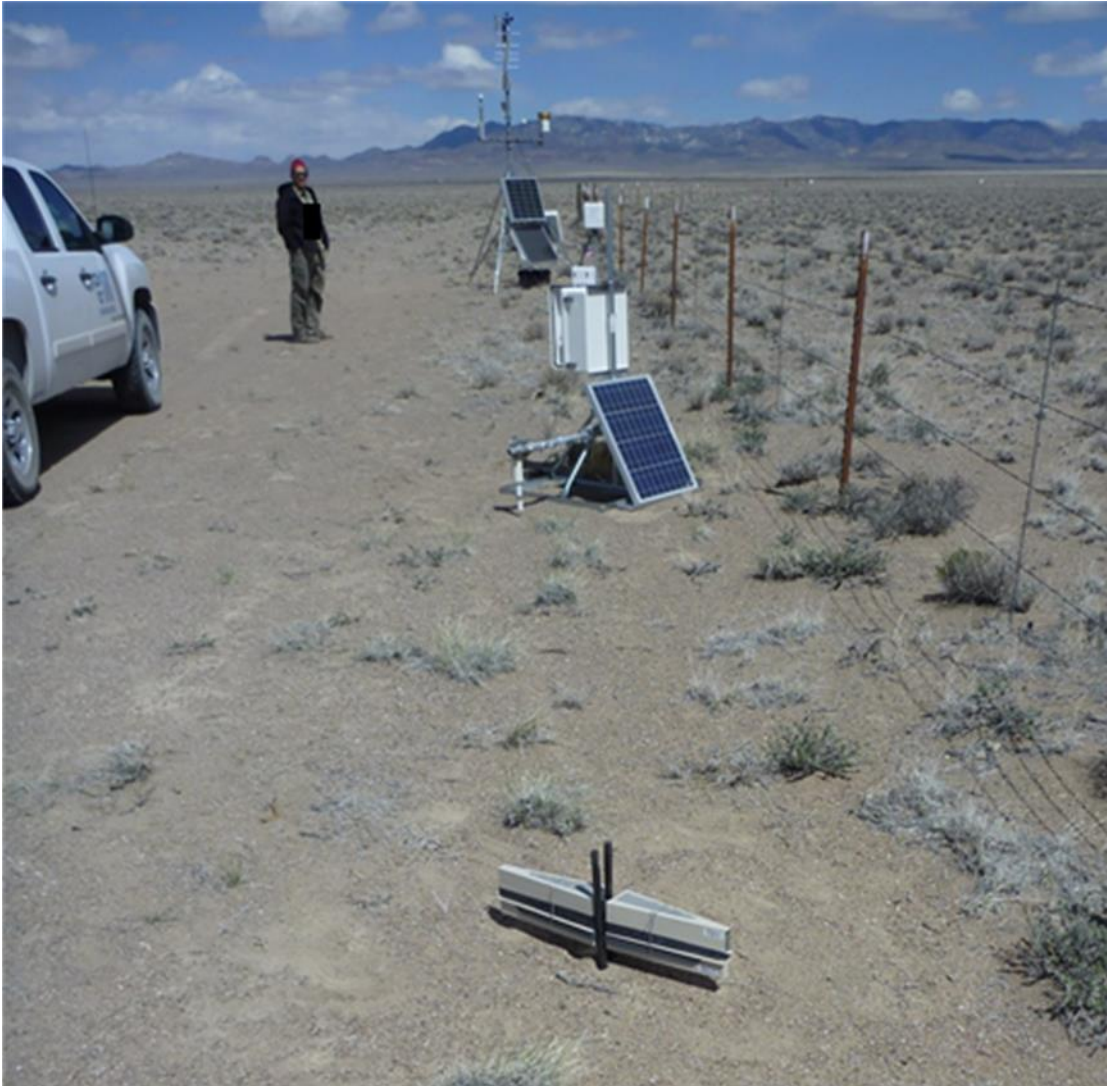
Figure 16. Typical installation of BSNE saltation traps. Photos for the Project 57 installations are not available, but this photograph taken at Clean Slate III (monitoring station 401) shows the type of installations used at Project 57. The BSNE saltation trap in the foreground is oriented with one opening facing the dominant wind direction coming across the fenced site to the right, and one facing away from the fenced area.
