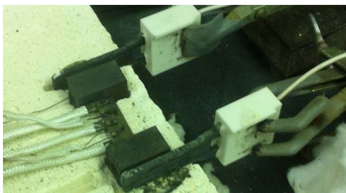
Figure 3-10 Thermocouples on the sample.
