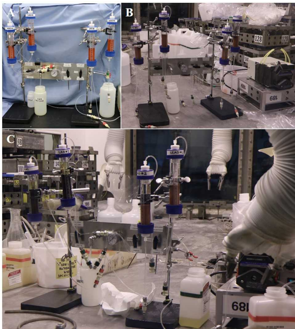
Figure 3-3. Ion Exchange Column and Manifold System.
