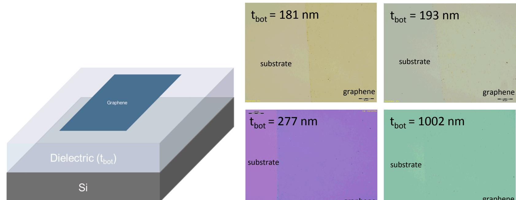
Graphene only absorbs 2.3% of light, thus is practically transparent. However, when placed on a dielectric, its contrast against the dielectric varies significantly. The contrast of exposed graphene on top of various dielectrics has been studied extensively but the same is not true for dielectrically encapsulated graphene. Here we aim to study the visibility of graphene when sandwiched between two dielectrics and show that the top dielectric layer can be tailored to vary the graphene visibility.
