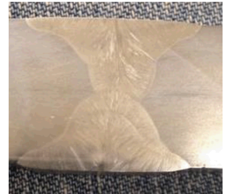
Weld zone, 304 SS plate. Photo: Ranor
