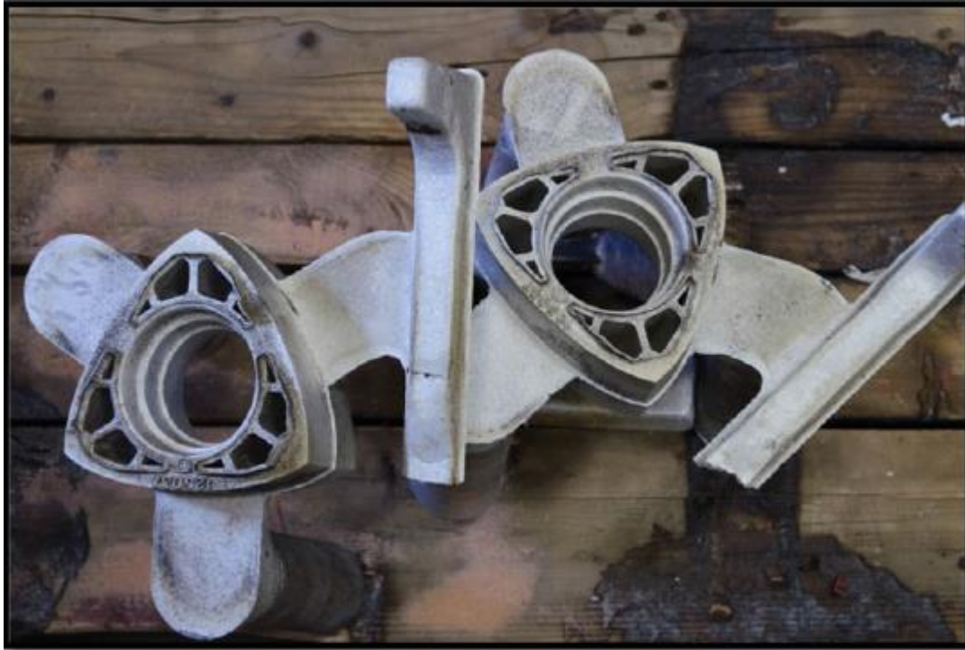
Figure 7: Rotary engine rotor castings produced in Al-8Ce-10Mg alloy.
