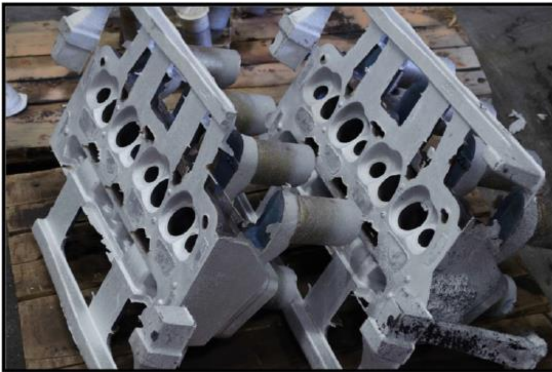
Figure 6: Automotive cylinder head castings produced in Al-8Ce-10Mg alloy.
