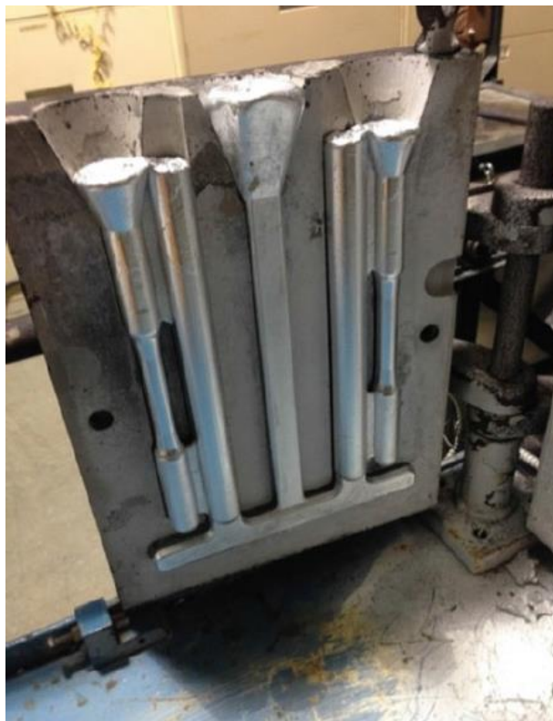
Figure 2: Partial fill test bar mold with Al-16Ce
