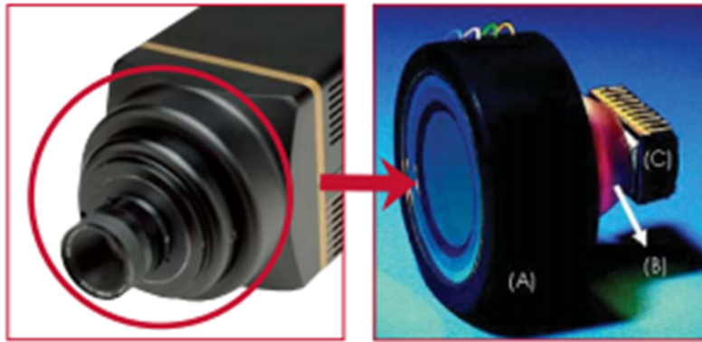
Figure 8. PI-Max ICCD camera showing image intensifier (A), fiber optic face-plate (B), and CCD (C).
