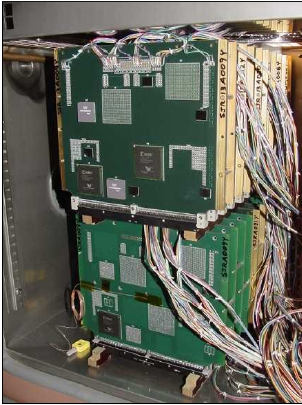
Test vehicles: wired and stacked in the thermal cycling chamber.
