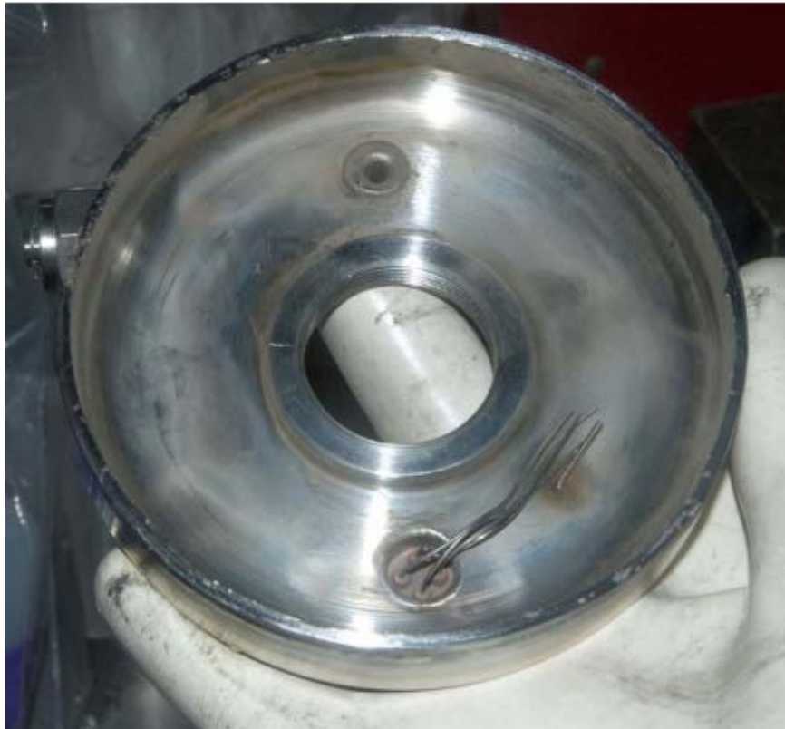
Figure A1-3. Modified inner 3013 container lid showing no corrosion after MB container loading: 105 days in surveillance.
