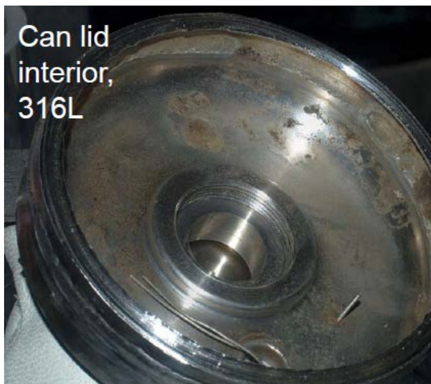
Figure A1-3. Lid from third modified inner 3013 container loaded with PMAXBS (0.4 wt% moisture, 100 days in surveillance). Corrosion observed throughout headspace region.
