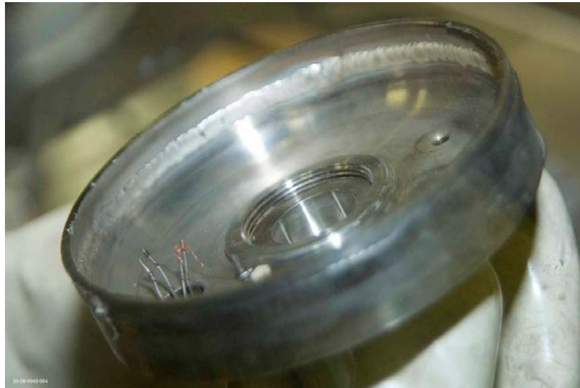
Figure A1-2. Lid from second modified inner 3013 container loaded with PMAXBS. Container reloaded with PMAXBS (0.23 wt% moisture; 400 days in surveillance) after leak was discovered in first container. Very slight corrosion observed in heat affected zone surrounding weld.
