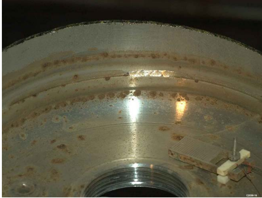
Figure A1-1. Lid from first modified inner 3013 container loaded with PMAXBS (0.19, 0.23 wt% moisture; 400 days in surveillance). Corrosion observed throughout headspace region.
