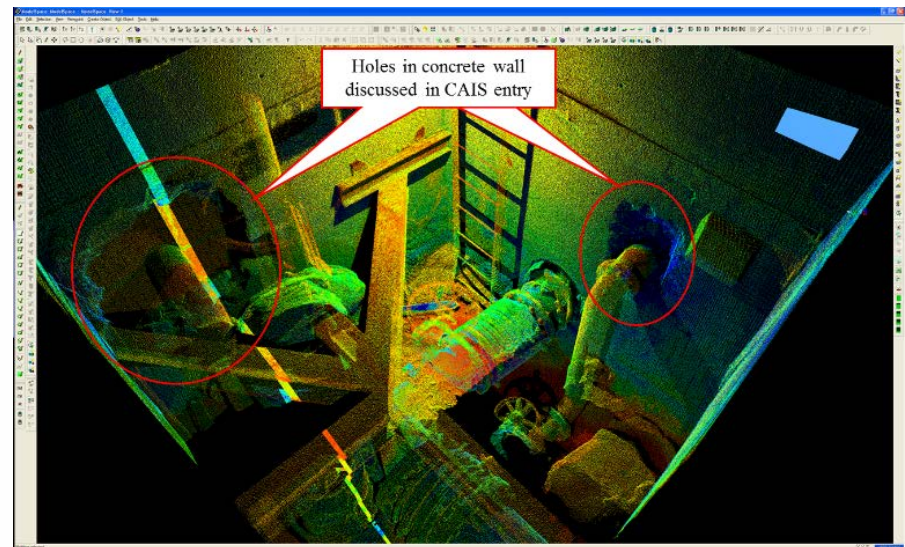
Example steam system thermographic inspection and steam pit LIDAR survey
