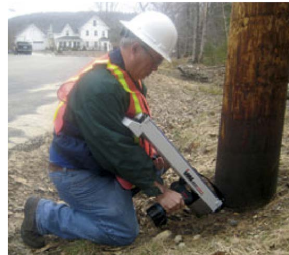
Example of wood pole micro-bore integrity inspection
