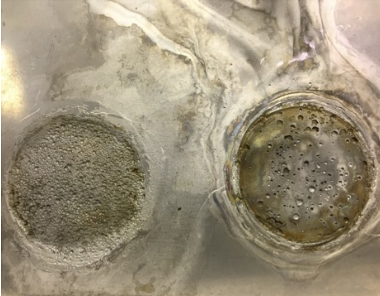
3M \text{FeCl}_3 Hexahydrate (left) - 7 day immersion vs. 1.5 M Anhydrous \text{FeCl}_3 (right) - 2.5 day immersion
