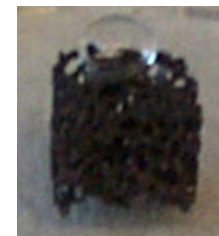
Contact angle > 120° on porous material
