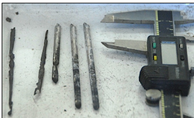
FIG. 2. U-TRU-Zr pins simultaneously cast in the GACS (calipers set at 25.4 mm).
