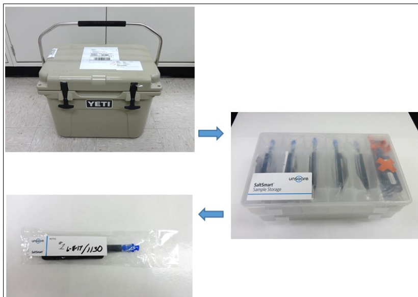
Figure 1. Packaging of SaltSmart™ samples delivered to SNL. Dry dust sampling heads (not shown) were packaged in the same manner.
