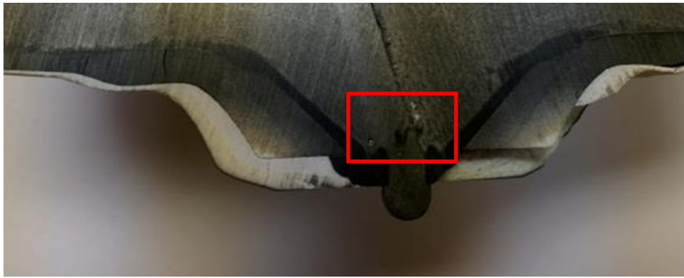
Figure 9: Cross section crucible at orifice showing area of tungsten agglomeration (Fig. 10) Scanning electron microscope images with EDS scans showed clumps of tungsten particles that agglomerated gadolinium oxides to the bottom of the crucible. These solid agglomerations appear to block the melt flow at the orifice (Fig. 10).
