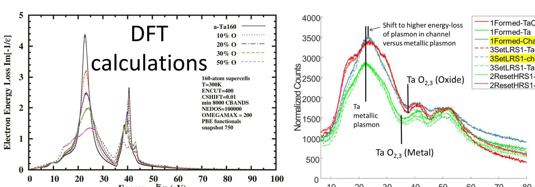
In filamentary region, Ta O<sub>2,3</sub> edge is consistent with oxidized Ta but there is a sharp metallic plasmon feature shifted to slightly higher energy loss consistent with DFT calculations for more metallic oxides
