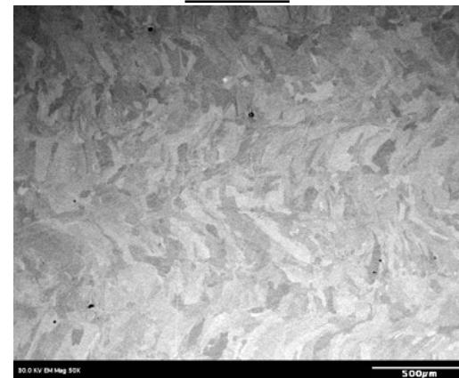
Fine solidification cell due to interpass boundary pinning
