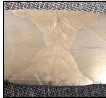
Weld zone, Ranor 304 SS plate
