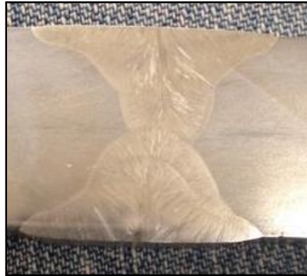
Weld zone, Ranor 304 SS plate
