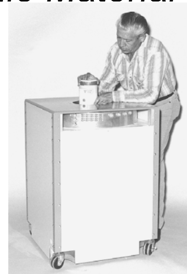
Plutonium Scrap Multiplicity Counter, used for accurate assays of plutonium metal, oxide, mixed oxide, or scrap (LANL PANDA Manual ).
