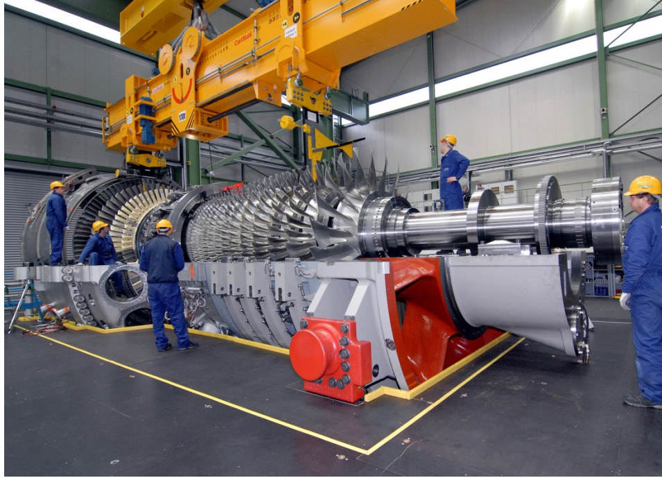
Figure 3. Siemens SGT5-800H rated at 375MW (similar to what used in the hybrid concept), located at the Siemens Berlin facility ready for shipment.
