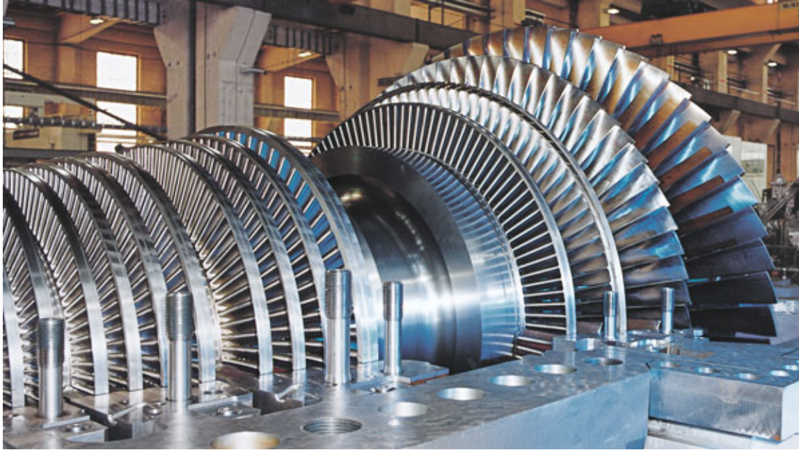
Figure 9. Steam turbine Siemens SST-800 ( https://www.energy.siemens.com/co/en/fossil-power-generation/steam-turbines/sst-800.htm#content=Description ).
