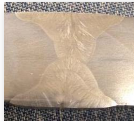
Weld zone, 304 SS plate. Photo: Ranor
