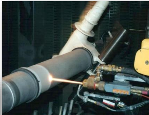
Hard Chrome Replacement on a Landing Gear Strut
