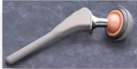
Hydroxyapatite coating on a hip implant
