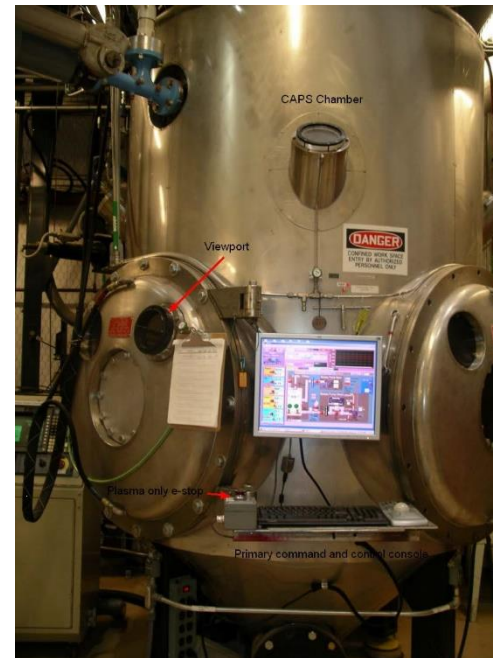
Vacuum, low pressure, and very low pressure plasma spray
