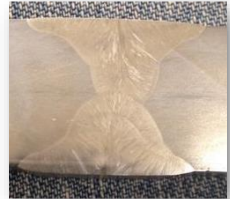
Weld zone, 304 SS plate. Photo: Ranor
