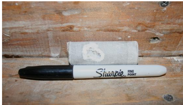
Figure 6-40: Full core plug sample from lower Little Falls Formation at depth of 6,355 ft showing saddle-shaped dolomite-lined vug.
