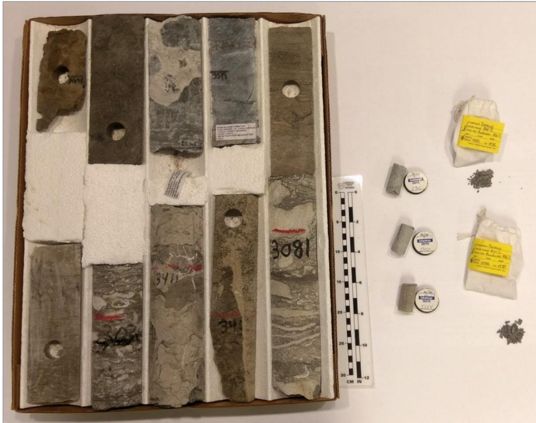
Figure 5-1: Conventional whole core, sidewall core, and drill cutting rock samples.
