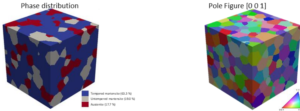
Figure 13: Hypothetical 3-D representative volume element for a hypothetical Q&P steel (RVE2)
