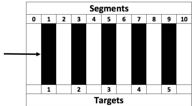
Fig. 3: Simple illustration of the MINERvA detector. There are five main targets of interest of differing metal compositions. Segments as defined by the target regions are the regions between the targets and the regions up and downstream of the targets.
