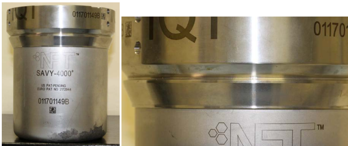
Figure 17 Exterior of SAVY 4000 after 47 hours of exposure to boiling MgCl_2 .
