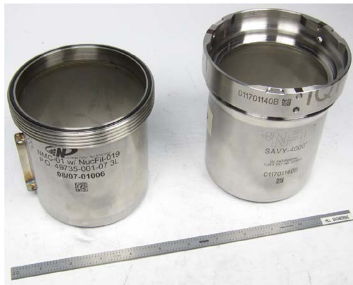
Figure 21 Photograph of the SVY and Hagan containers used for hole drilling measurements
