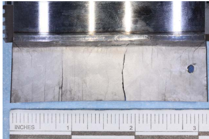
Figure 6 Inner contour of the Hagan-1 section after 16 hours of exposure to boiling MgCl 2 .
