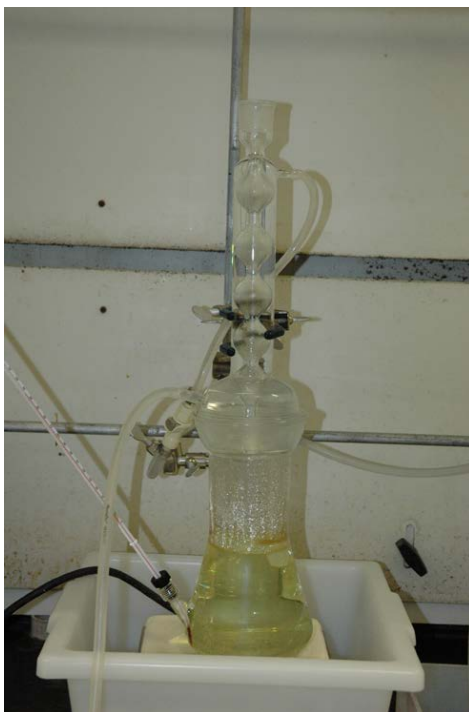
Figure 4 Experimental set-up for the boiling MgCl_2 experiment on container pieces.
