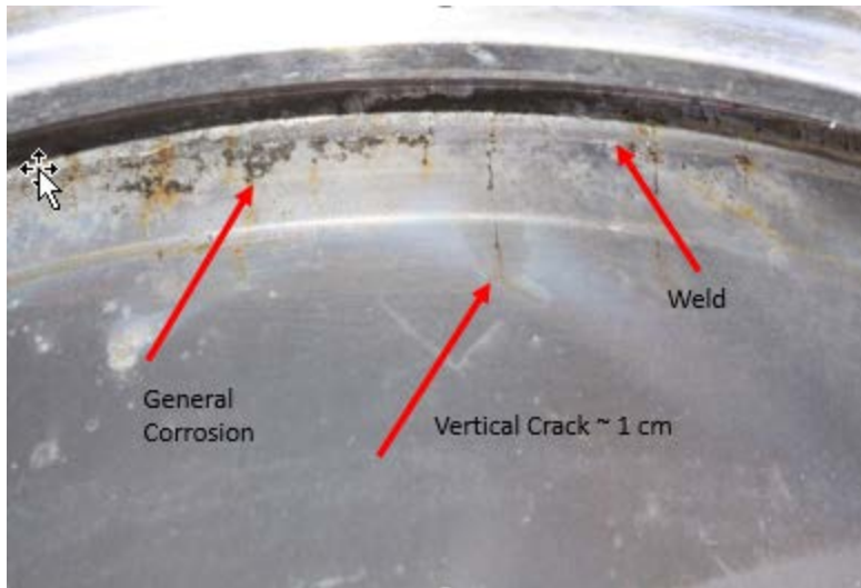
Figure 19 SAVY 4000 inner wall weld region after exposure to boiling MgCl_2 showing vertical cracks and general corrosion.
