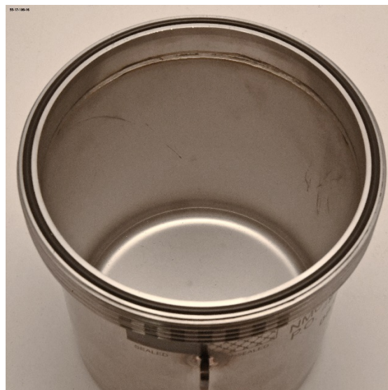
Figure 11 a) Exterior and b) interior of the one quart Hagan container prior to exposure to boiling MgCl_2 .
