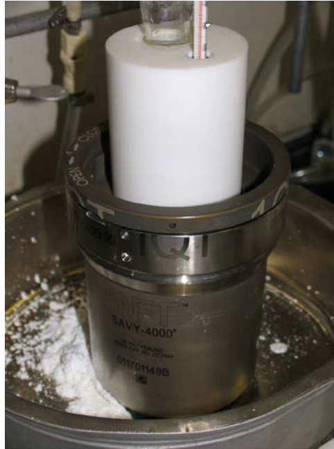
Figure 14 SAVY 4000 container after failure with MgCl_2 in catch pan.
