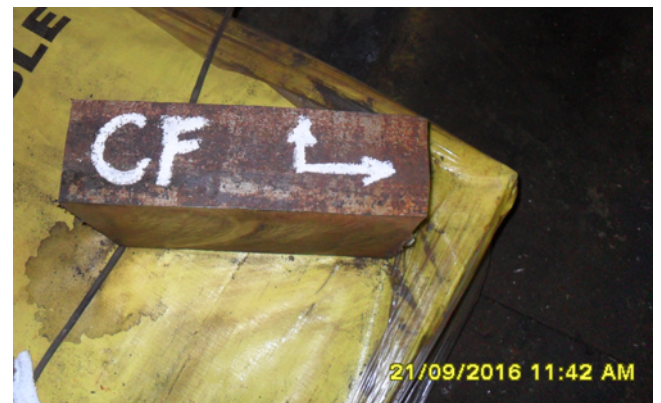
Fig. 15. CF block with orientation marked (Y axis is perpendicular to the beltline weld with the arrow pointing to the top of the segment and the X axis is parallel to the weld with the arrow pointing to the right of the segment) [15].
