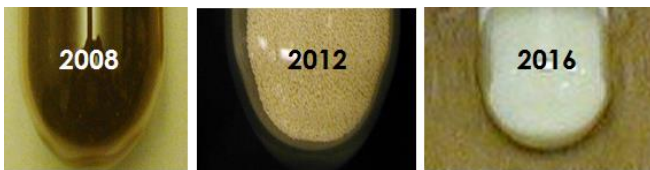
Figure 2a. Commercial samples of as-received \text{EuI}_2 feedstock. Over time, vendors have improved purity and stoichiometry.
