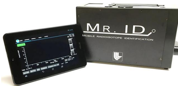
Figure 1b. Prototype radioisotope identification detector engineered by Lawrence Livermore National Laboratory, incorporating a 1.5" x 1.5" SrI 2 (Eu) crystal, and the radioisotope ID software, "RNAK" [18].
