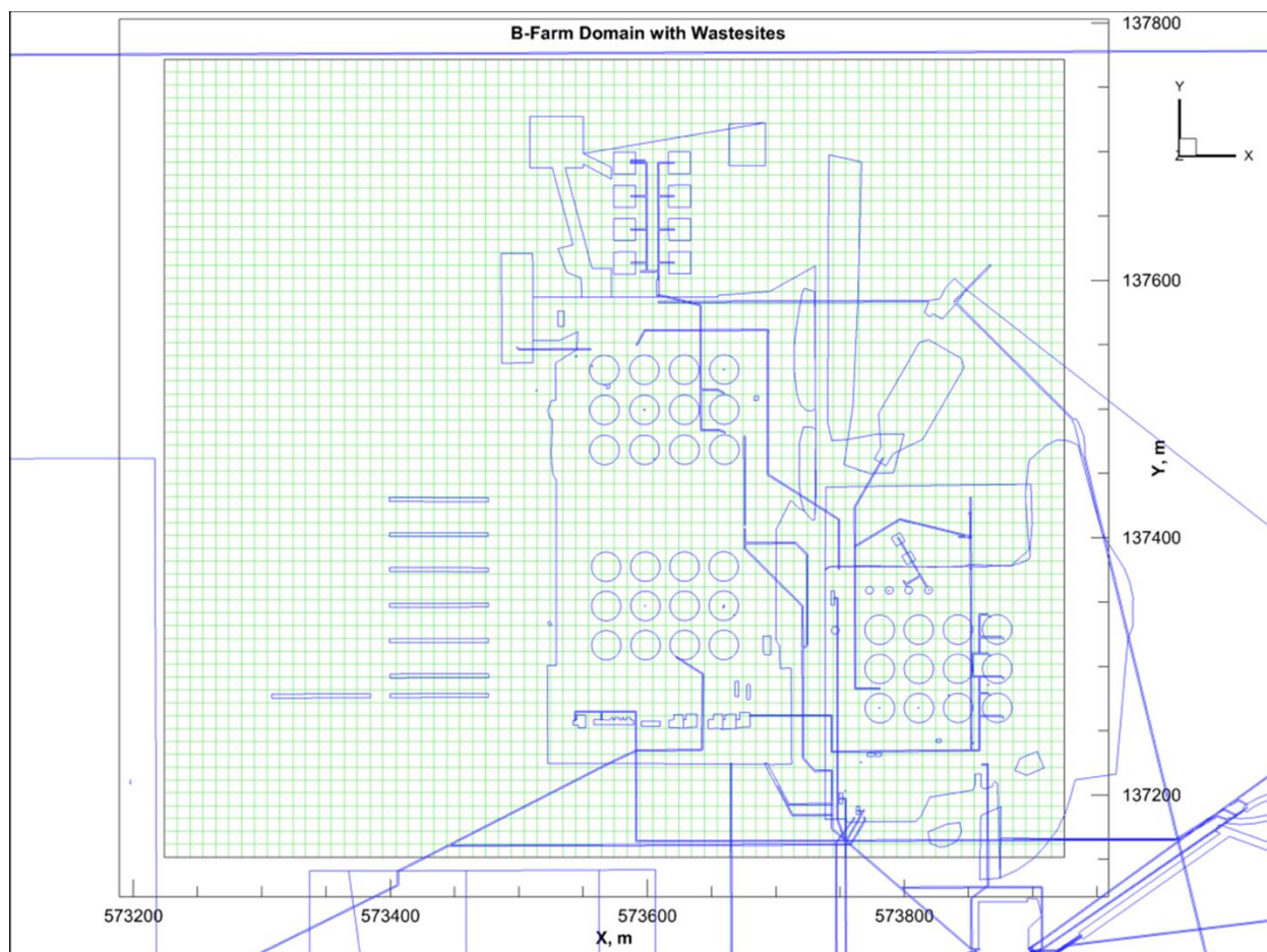
Figure 18. Plan-View of a Preliminary Model Grid with Waste Sites Superimposed for Source Term Mapping
