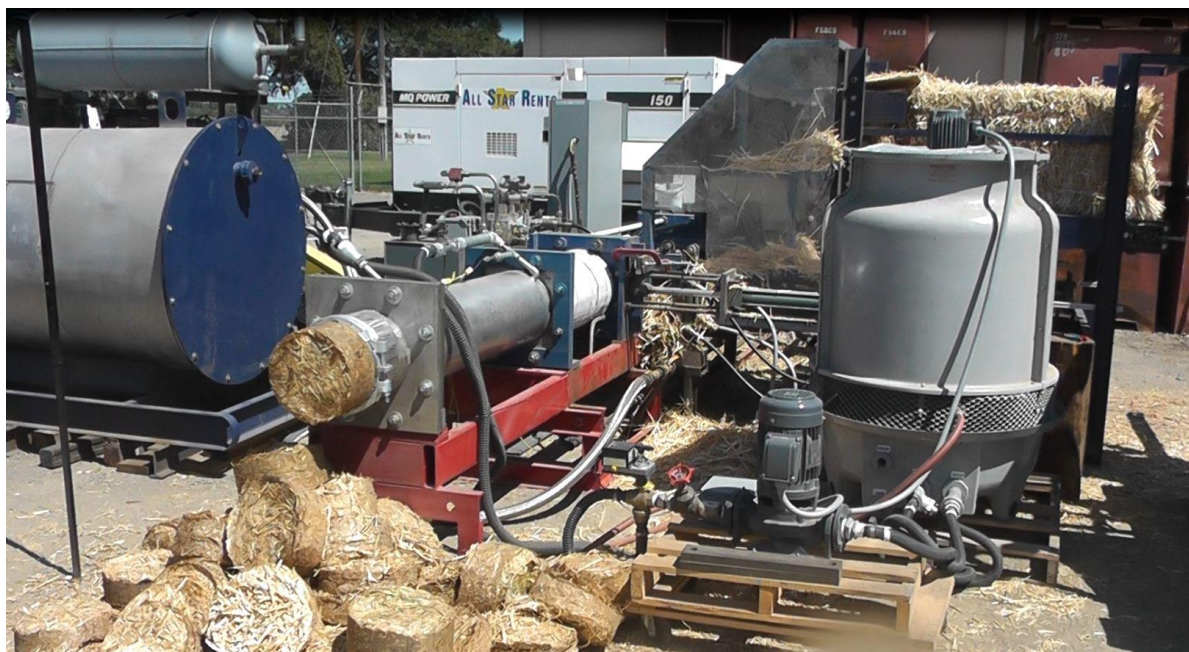
Figure 1. The BBADS equipment that is part of the GHGR-CBTL full scale plant for densifying the feedstocks to minimize the feedstock transportation cost and energy.
