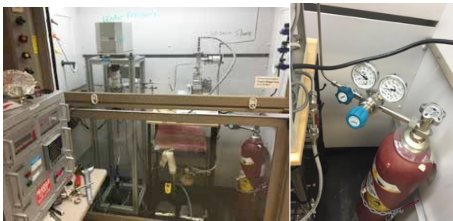
Figure 19: Photographs of Rubotherm gravimetric microbalance system in hood to determine the effect of SO 2 and NO x on NDIL0230, NDIL0309 and encapsulated versions of these materials.
