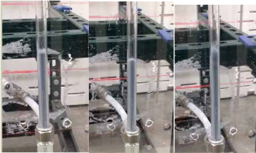
Figure 56a: Pictures of fluidization of polyethylene spheres at gas flow rates of 1.0, 2.0 and 3.0 l/min.
