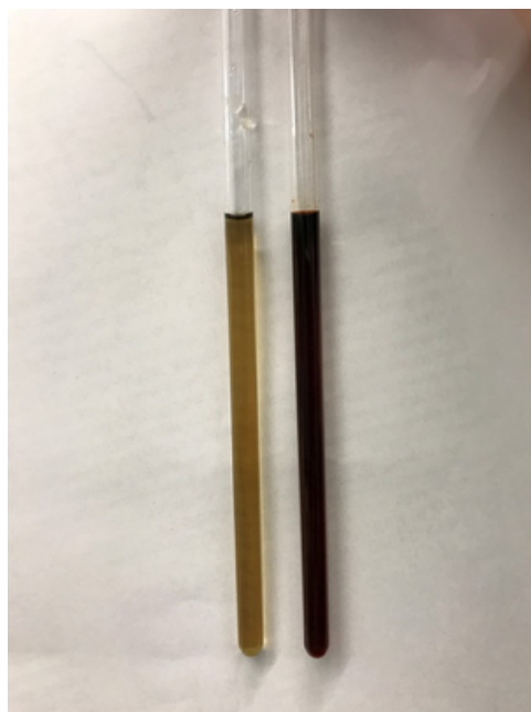
Figure 21: The color of the NDIL0230 changed after exposure to NO. The left NMR tube is pure NDIL0230 in DMSO. The right NMR tube is the NDIL0230 after exposure to NO, followed by pulling vacuum, in DMSO.
