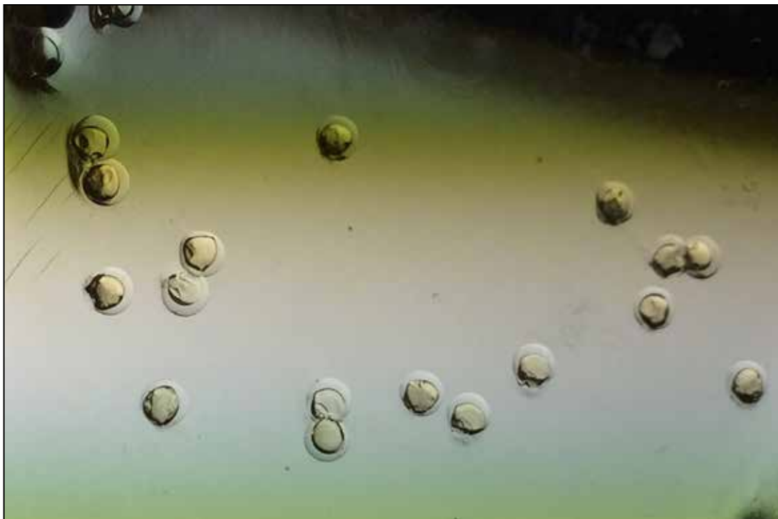
Figure 41: Photo of preliminary NDIL0230 (100% neat IL)-Thiolene-Q (TPO-L) capsules generated with IDEA system.
