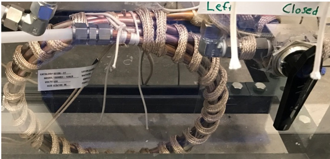
Figure 52: Preheater assembly – inlet loop.
