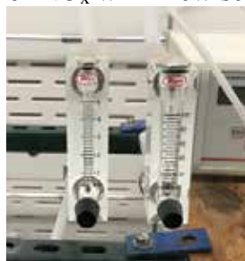
Figure 46: One set of rotameters that cover up to 100 liter/min.
