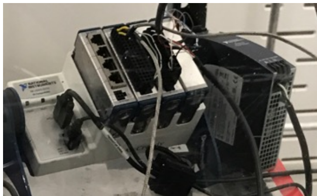
Figure 51: Interface module for thermocouples and pressure transducers.
