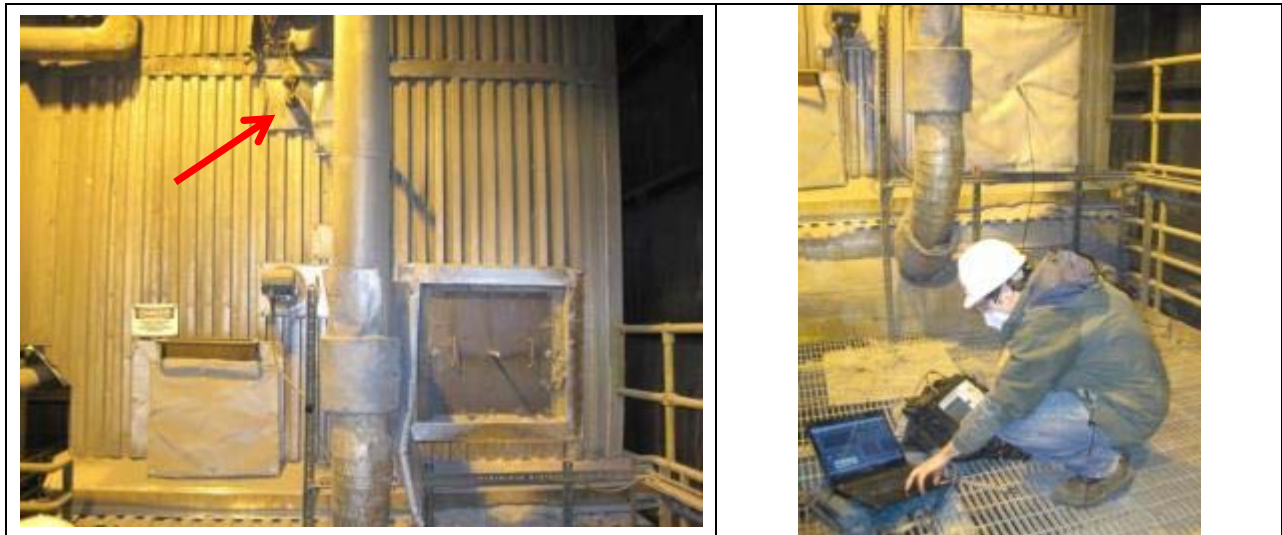
Figure 46: Left: sensor array panel installed at PERC. Right: Environetix engineer performing wireless interrogation tests with the six sensor array panel.
