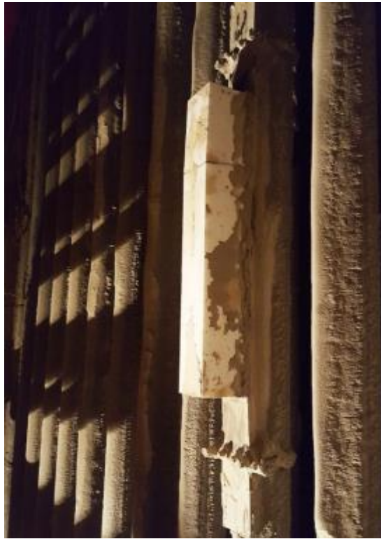
Figure 54: One sensor package retained a ceramic cover, but it was cracked, which compromised the sensor inside.
