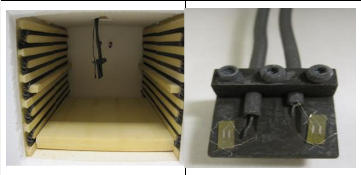
Figure 7: Box-furnace testing and typical fixture: (Left) SAW devices located inside the box oven; and (Right) LGS SAW resonator devices packaged on an Inconel plate.
