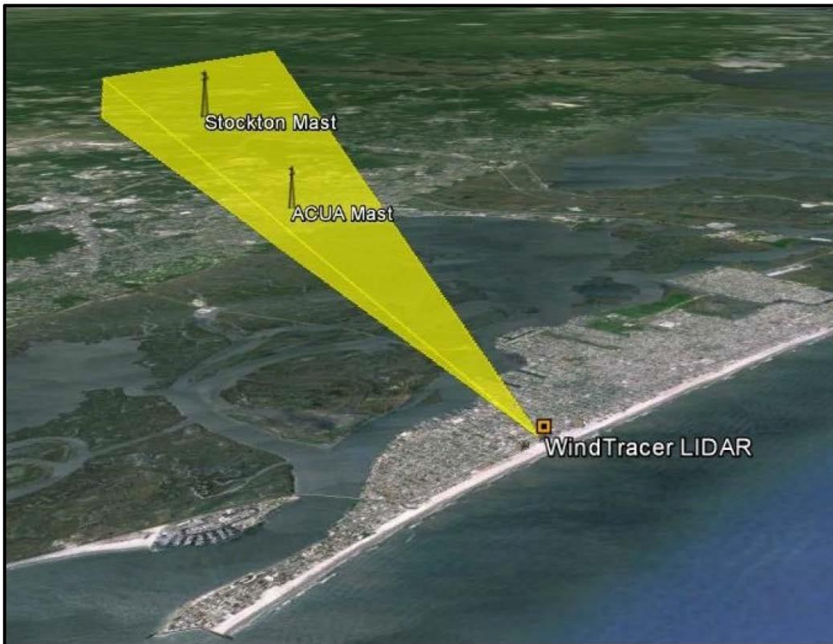
Figure 3. Depiction of the approximate LIDAR sampling volume at the ACUA and Stockton meteorological masts.
