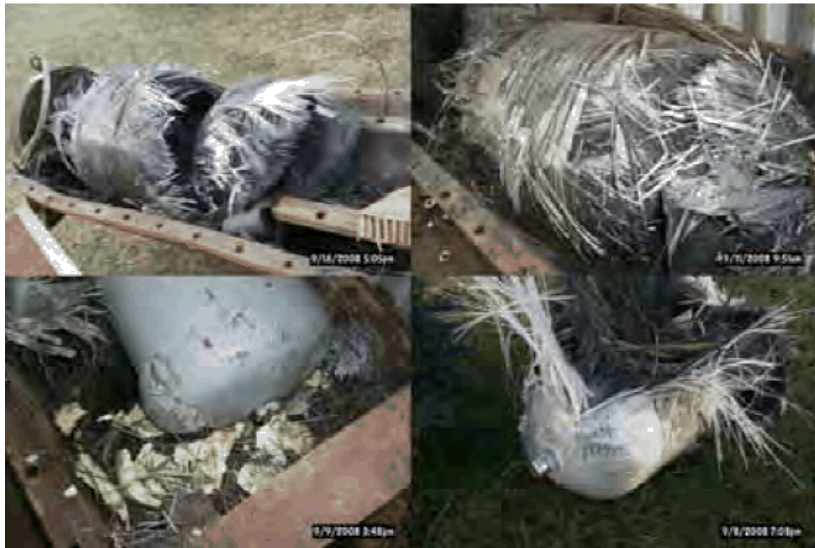
FMVSS 304 Hydrogen Cylinders Following Burst Pressure Test
