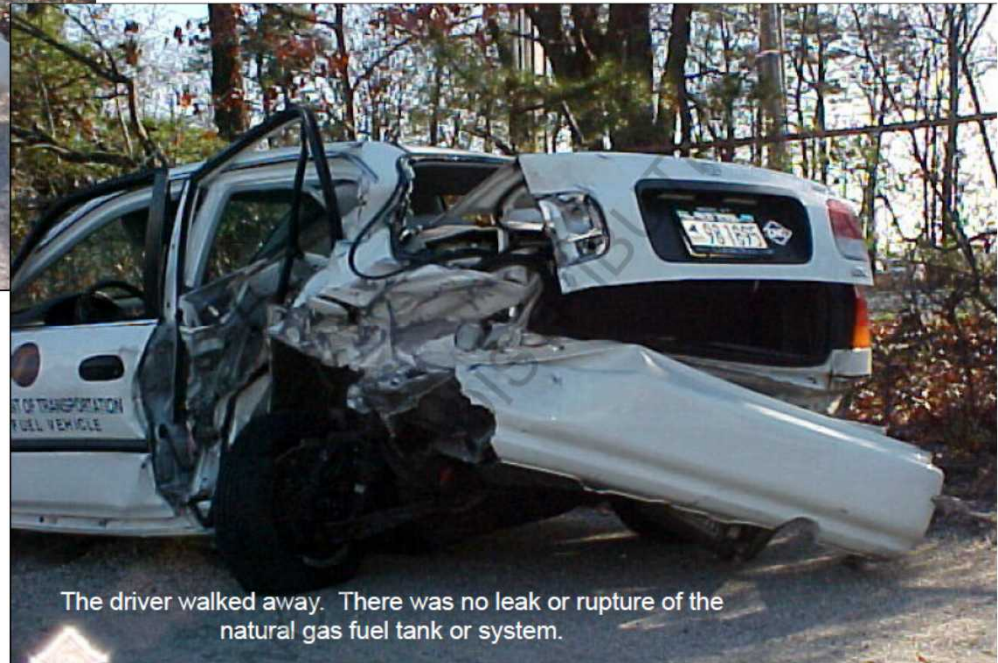
The Civic was crushed to the "B" pillar behind the driver's seat.
