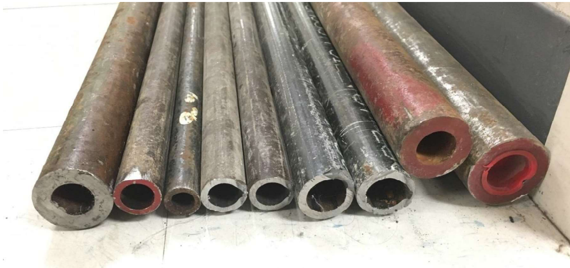
Figure 3-1 P91 pipes purchased for the FO-SHM system demonstration
