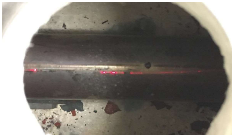
Figure 12-3 Fiber light leakage after a high temperature test
