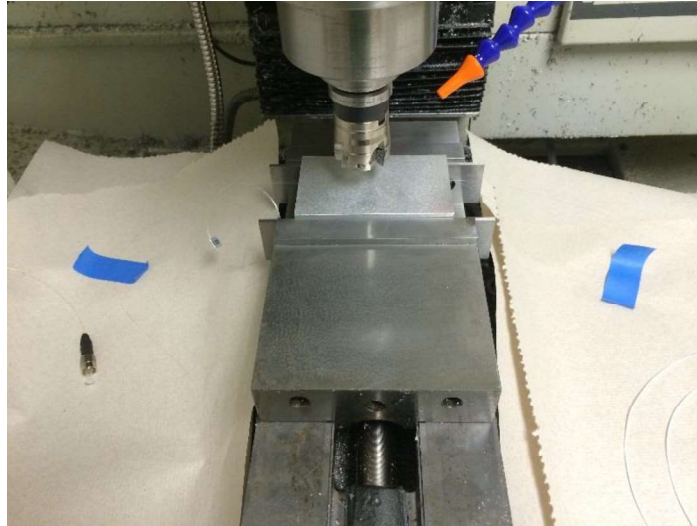
Figure 9-5 Milling off sample bottom to simulate the corrosion
