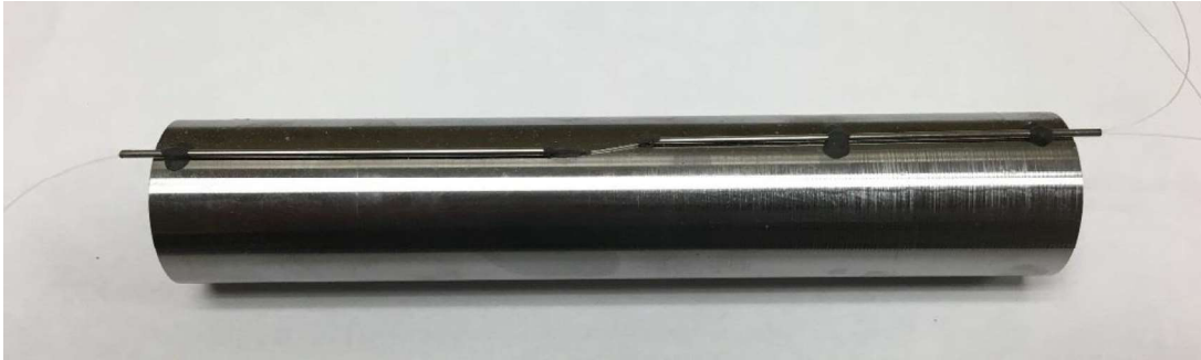
Figure 10-20 Completed state of the FO-SHM node on a P91 pipe
