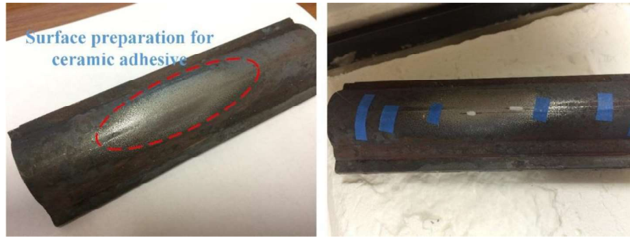
Figure 10-5. FO-SHM element surface attached to a P91 pipe by high temperature ceramic adhesive.
