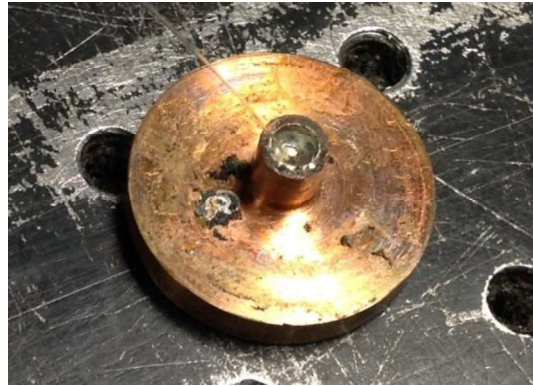
Figure 6-4. Demonstrative optical fiber LIP acoustic generating unit.
