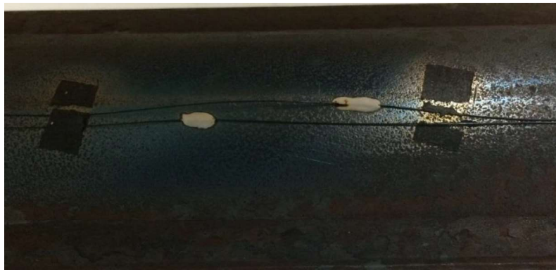
Figure 10-6 Surface attached FO-SHM element after the high temperature test
