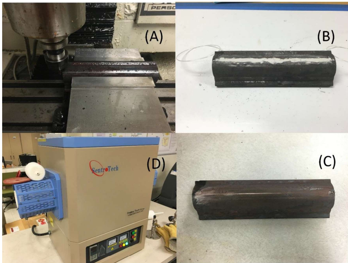
Figure 10-13 Full embedment sample preparation and new large volume tube furnace used in the test
