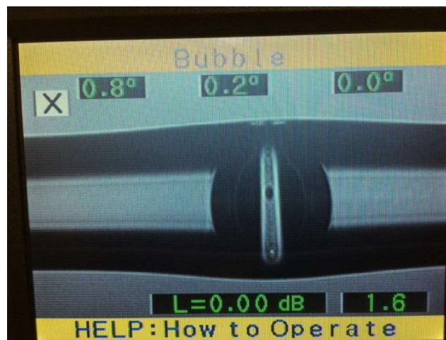
Figure 6-17. Improved splicing of the second LIP FO-AGU
