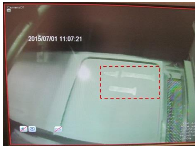
Figure 16. Short Feed during the Building Mechanical Test Walls from S1-F Powders (the dashed line shows the area with short-feed)
