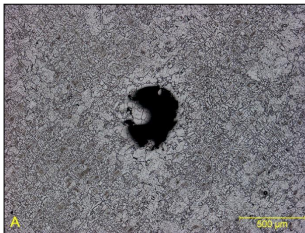
Figure 25. High Magnification Imaging of Macrostructure in the NIST Test Artifact Produced with the S1-F Powder (the hole has a nominal diameter of 0.25 mm)
