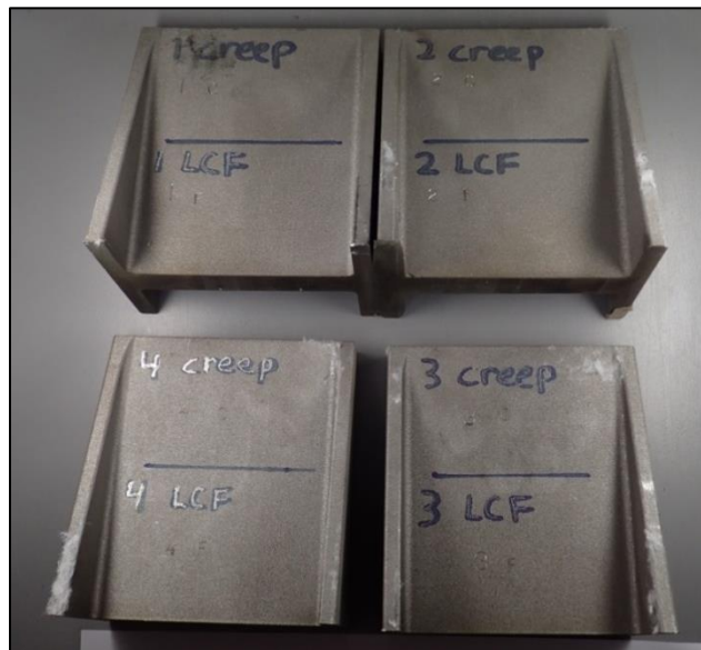
Figure 79. Mechanical Test Walls Produced for the Fabrication of Creep and Fatigue Specimens along the XY Direction
