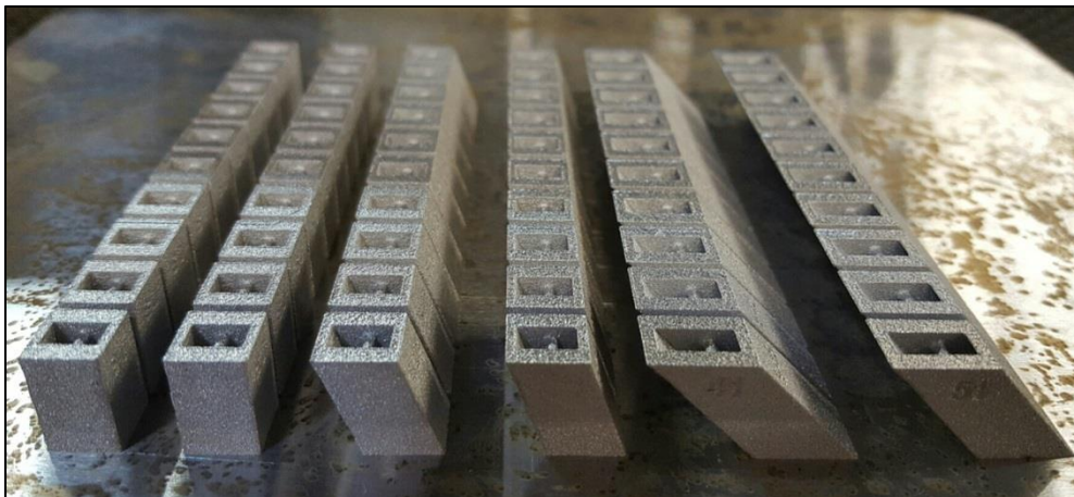
Figure 100. Specimens Produced with Three Inclination Angles of 0, 20, and 45 Degrees for the Analysis of Surface Roughness and Dimensional Accuracy
