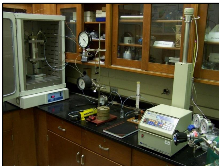
Figure B.8: Set-Up of the Triaxial Core Holder and Syringe Pump for Measurement of Changes in Permeability of Plug 2FD-1 while Exposed to NaCl Brine and Solution of CO 2 in Brine
