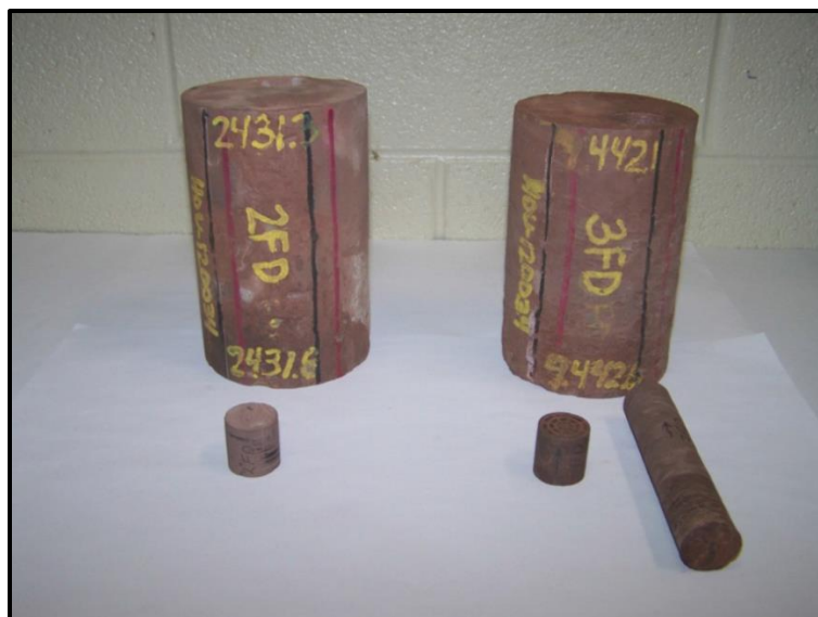
Figure B.1: Four-Inch Diameter Cores 2FD and 3FD from Well D-9-9 No. 2 in the Citronelle Field
