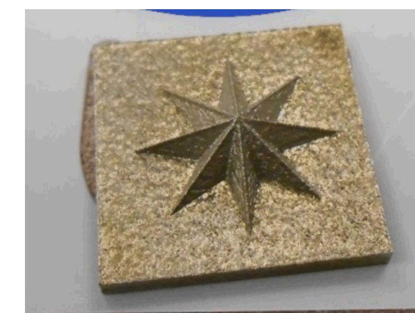
PH17-4 Siemens star produced by laser powder bed fusion
