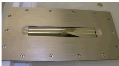
Figure 13. WC/SiC multilayer coated cylindrical glass segment in coating fixture
