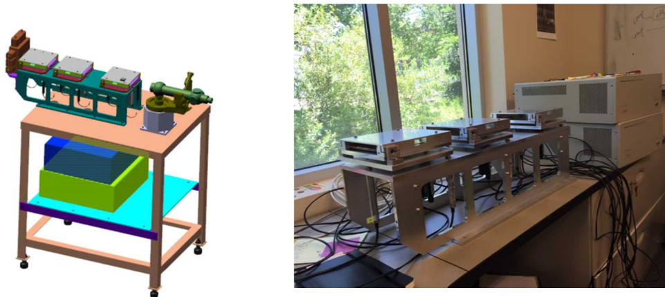
Figure 7. Rendering of the three-mirror optics with JJ-Xray slits -the real set-up includes a W collimator- and alignment scope (left). Three-mirror system (right). Plates on top of mirror holder are removed during experiment.
