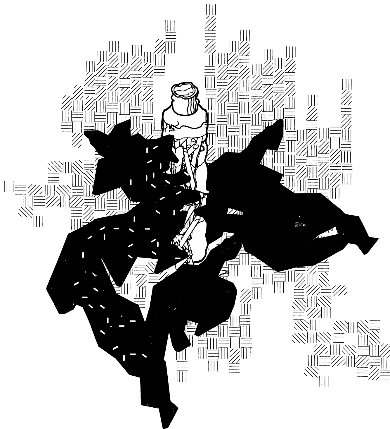
Sketch 12-2. Magma reaches container through small connected fractures and carries away contaminant debris from the container.
