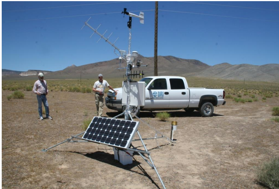
Figure 3. The Smoky CA meteorological station was installed to measure precipitation, wind, and other climate parameters.
