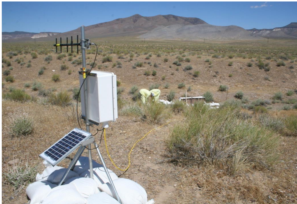
Figure 5. Runoff conditions in the flume are detected by the pressure transducer (yellow cable), recorded in the datalogger (white box), and relayed by radio (black antenna) to the meteorological station for transmission to the WRCC via the GOES.
