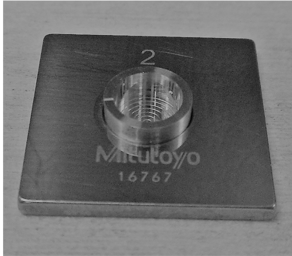
Fig. 6. Copper thickness standard glued into 2mm gage block with alignment notch visible.
