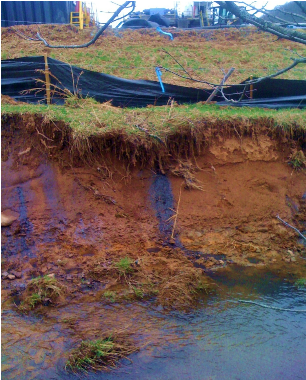
35. Photograph of a black substance identified as drilling mud oozing out of the ground from an eroded stream bank below a drill pad and into the water of Indian Run in Harrison County, West Virginia, in 2010. Photo by Doug Mazer, used with permission.
