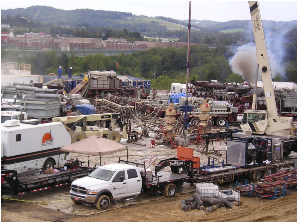
25. Photograph showing a hydraulic fracturing operation in progress on a Marcellus Shale well in Greene County, Pennsylvania. Photo by Dan Soeder in 2011.
