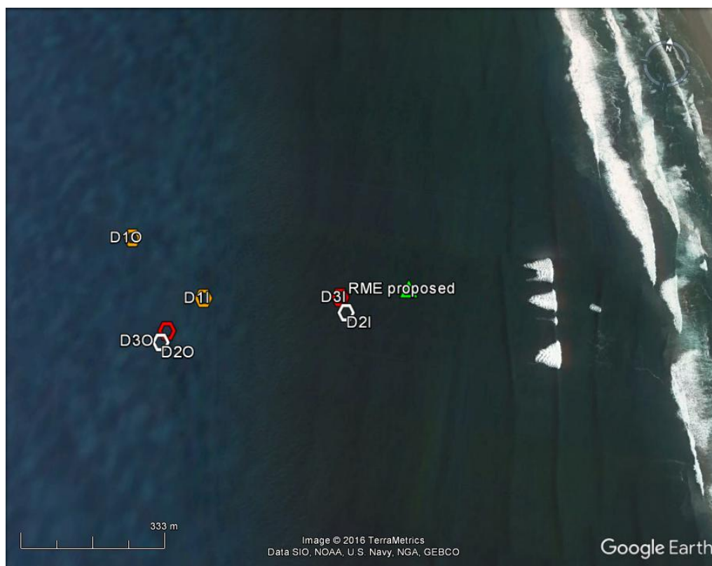
Figure 1. The color coded deployments (D1 orange; D2 white; D3 red) and locations of the inshore (I) and offshore (O) hydrophone landers at Camp Rilea, OR in 2016. The proposed location of the RME surgeWEC is shown as a green triangle shoreward of the landers.
