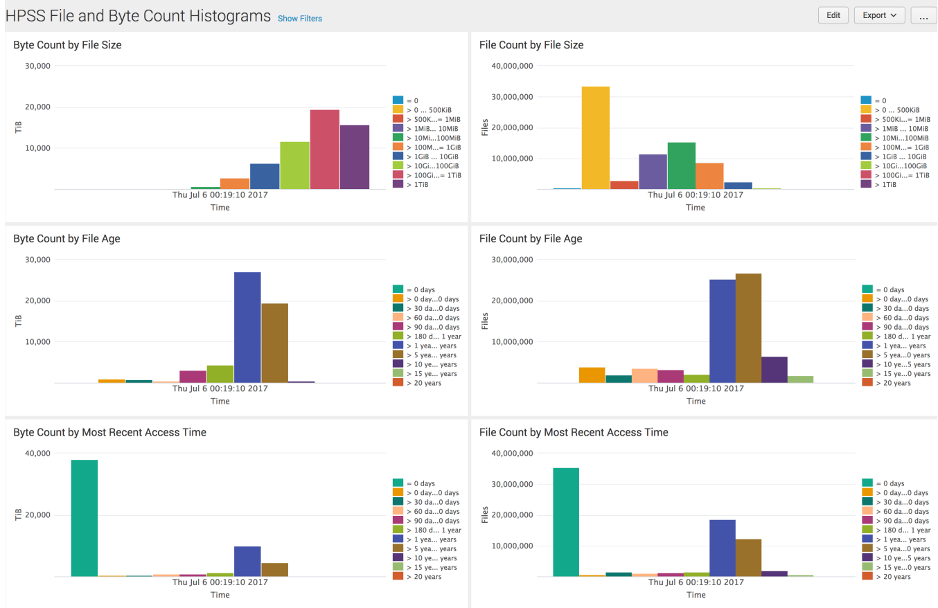
Figure 11: HPSS File and Byte Count Histograms as of July 6, 2017. The top two charts show the space occupied and number of files for each size range while the middle two show the space occupied and number of files for each age range. The bottom two charts show the space occupied and number of files sorted by their last access time (where "0 days" means the file has never been retrieved).
