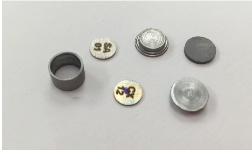
Fig. 8. "H-cup" piece parts and engraved sample coins.
