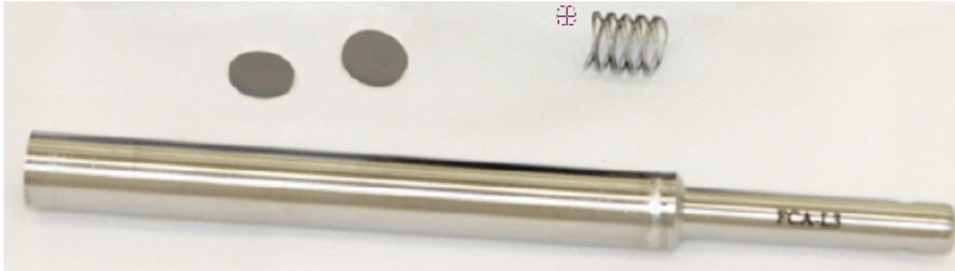
Fig. 6. FeCrAl steel capsule containment
