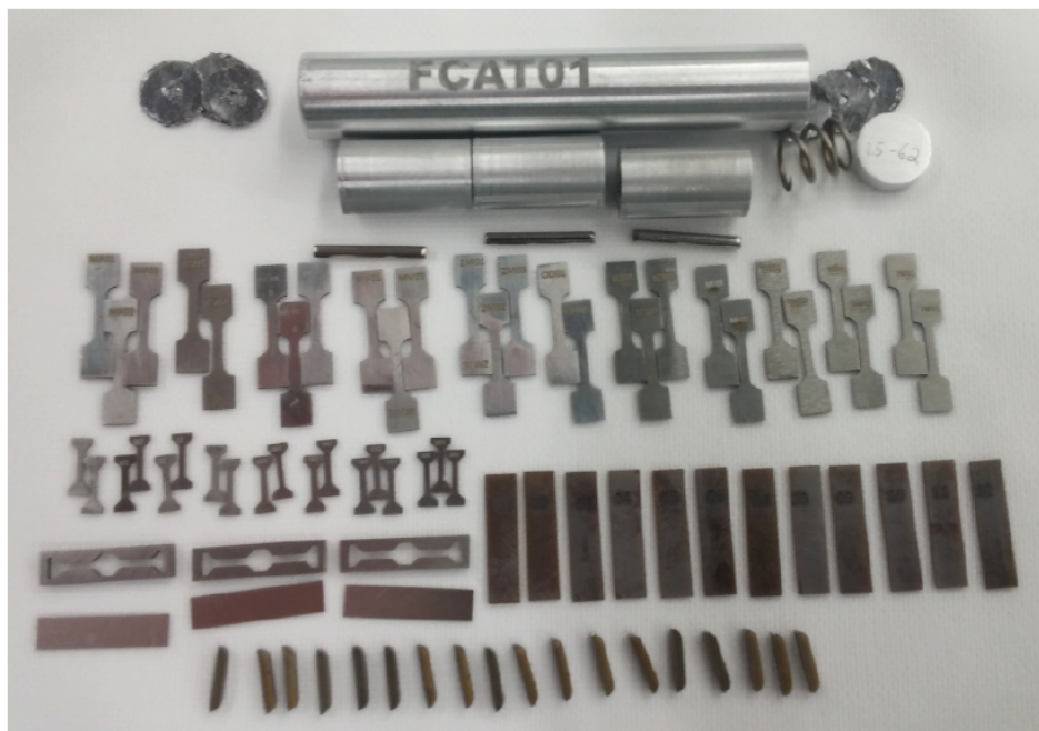
Fig. 2. Representative FCAT Capsule
