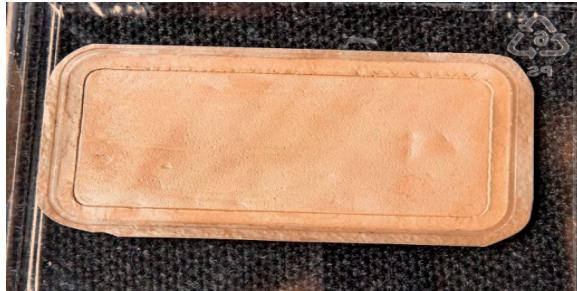
2"x4" GO/polymer membranes Month-long desalination tests show stable rejection
