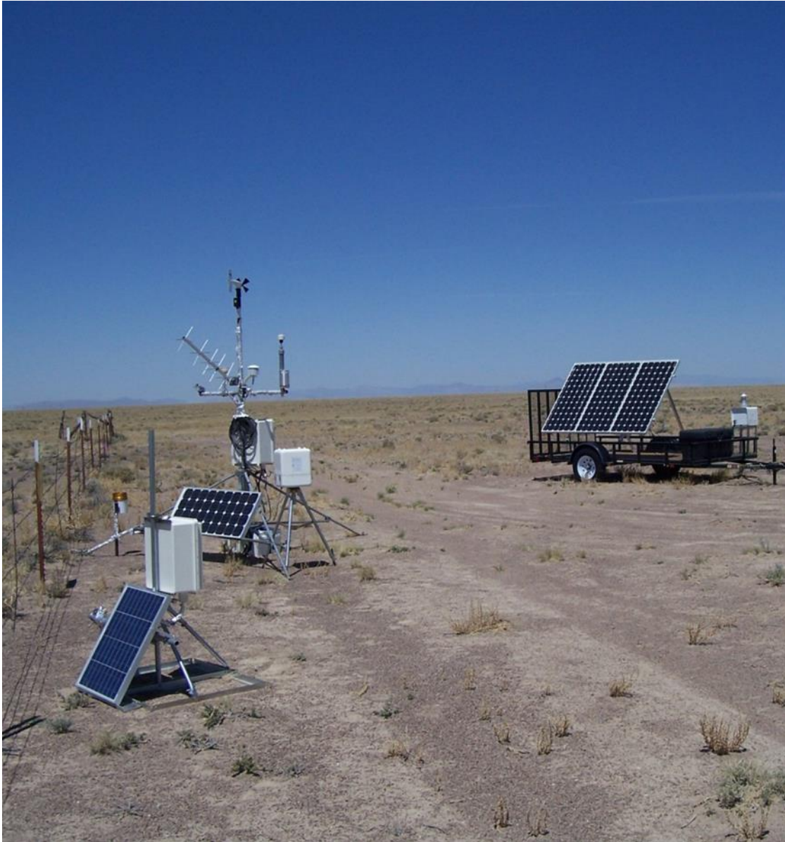
Figure 5. The solar powered air sampler, saltation sensor, and meteorological tower (center right, foreground left, and center left, respectively) at Station 402 are located along the north fence that bounds the Clean Slate I contamination area.
