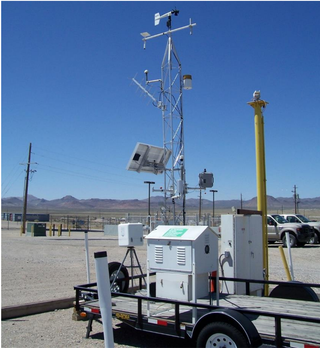
Figure 3. Station 400 is a trailer-mounted radiological and meteorological measurement system located near the Range Operations Center (ROC) in the Sandia National Laboratories (SNL) compound on the TTR.
