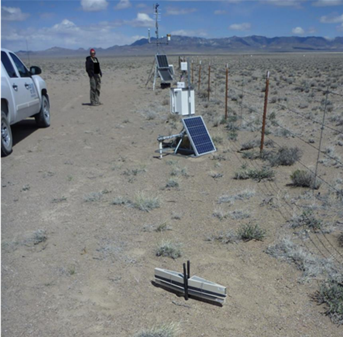
Figure 7. Northeast view at Station 401. In the foreground is one of three BSNE sand trap installations at TTR Clean Slate III. The Clean Slate III boundary fence is to the right. Behind the sand trap is the saltation sensor and meteorological station with additional sand traps located along the fence line.
