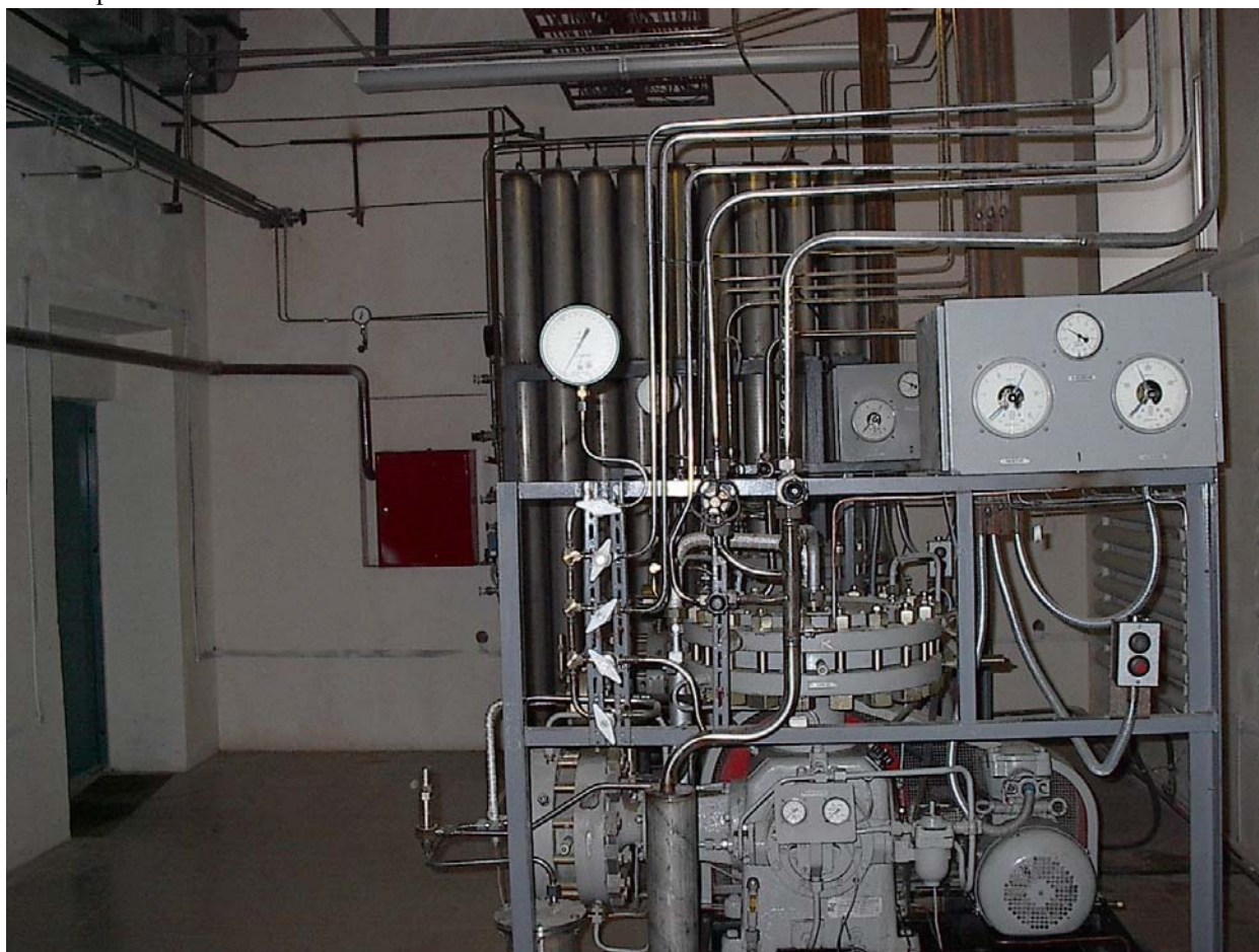
Picture 3: Pumps and gauges used to monitor and control the circulation of water vapor for the isotopic separation of O16 from O12.
