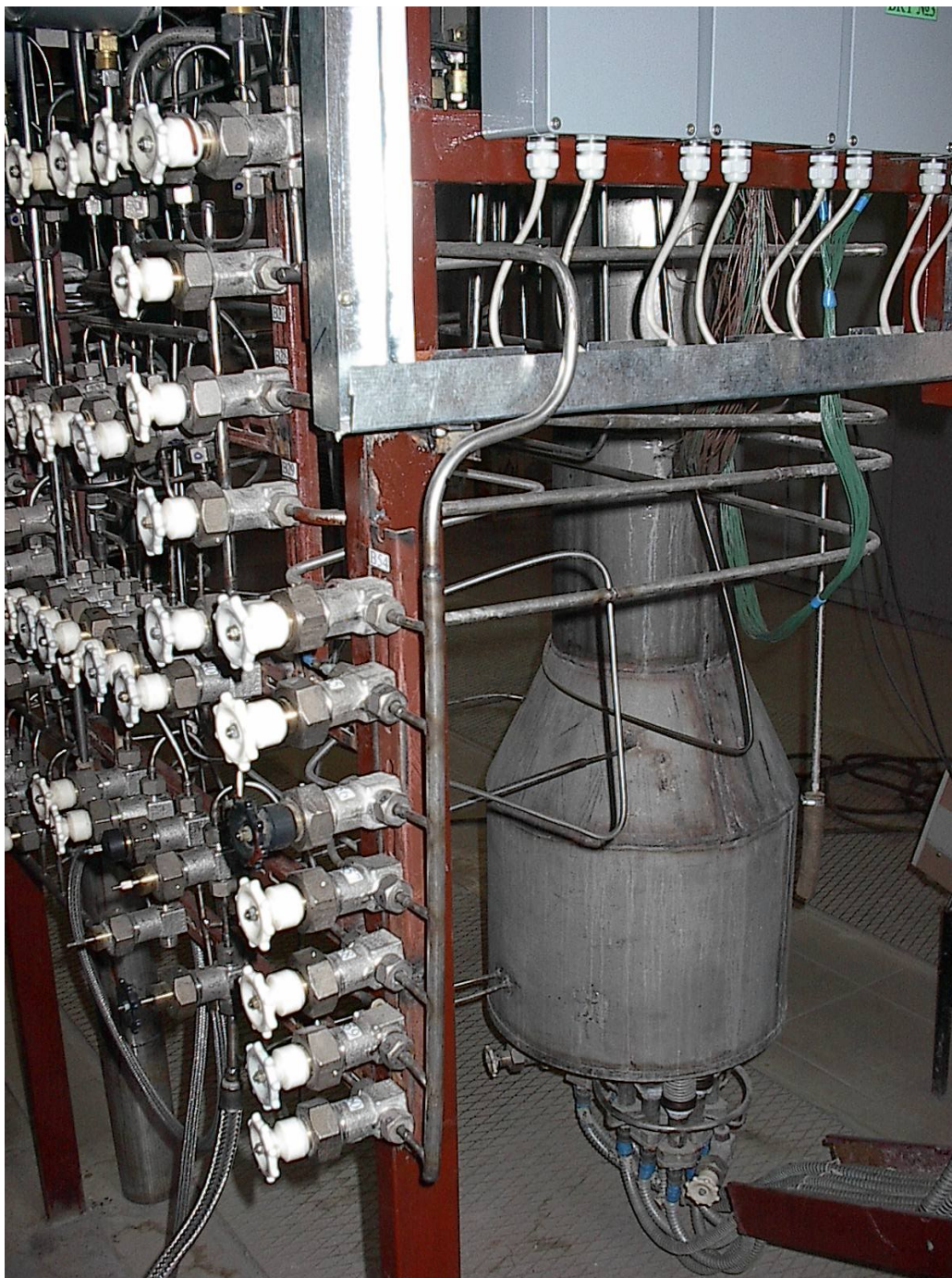
Picture 4: Water vapor condenser for the first stage of isotopic separation using the slight isotopically sensitivity of the rates of boiling between \text{O-16H}_2 and \text{O-12H}_2 to effect the isotope separation.
